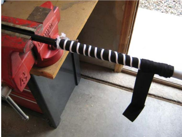
Figure 7. Wrap the hockey tape over the grip.
